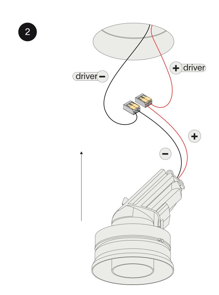
For serial connections, respect polarity.
