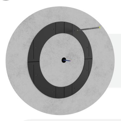
Once you've chosen the mounting location, use the provided **Hole Stencil** to accurately mark the drilling points. Ensure that the wires for connection are positioned centrally.
