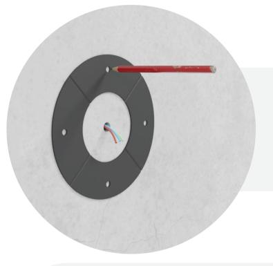
Once you've chosen the mounting location, use the provided 'hole stencil' to accurately mark the drilling points. Ensure that the wires for connection are positioned centrally.
