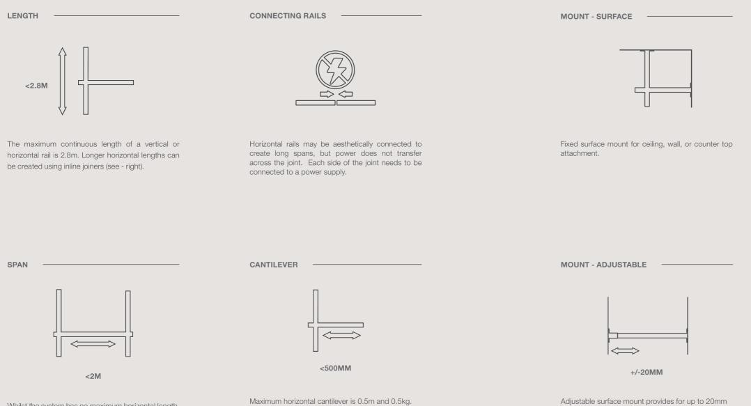
Whilst the system has no maximum horizontal length, the maximum distance between vertical supports is 2m.
