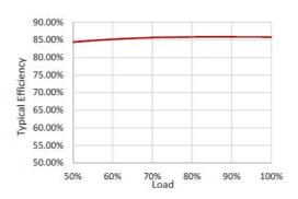
OT FIT 36 220-240 24 PC Typical Efficiency vs. Load
